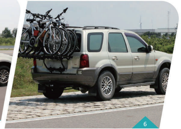
6. Belgium Blocks Test: Racks pass rough road test which means 6 km of driving over bumpy road.
