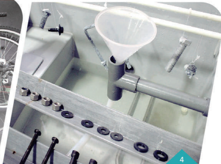
4. Resistance of Corrosion Test: Components are submitted to anti-corrosion test for 192 hrs at salt spray chamber.
