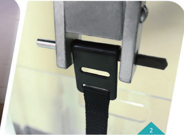
2. Universal Tensile Test: Textile straps with hooks are tested by pulling & breaking test.
