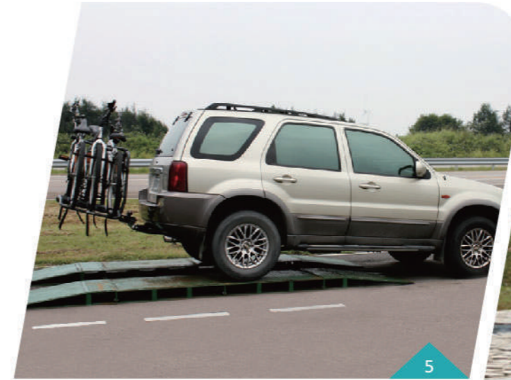
5. Sleeping Policeman Test: Racks pass ramp test which means three times of high speed driving test over a ramp.
