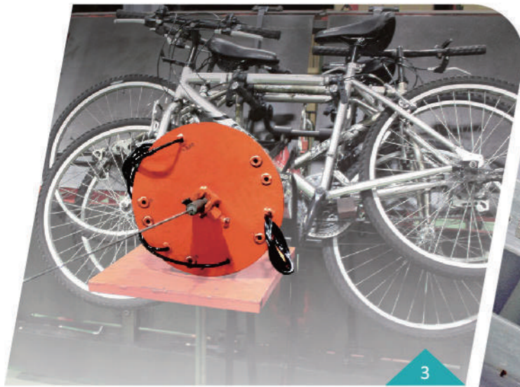
3. Breaking Test: Racks are tested up to four times of loading weight (250 kgs) at six directions.
